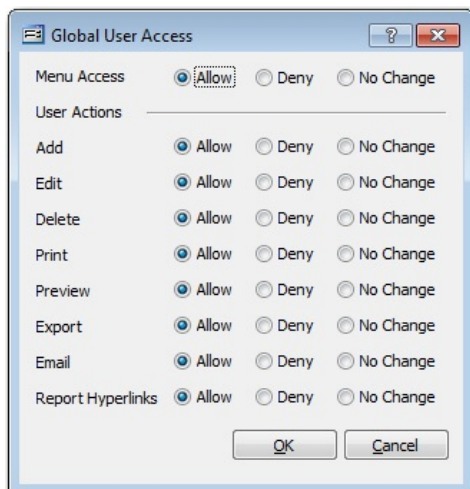
Figure: JB-84 Global User Access screen form showing the three types of access control for each form of access.
