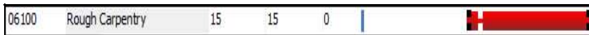
Figure: JS-80 Visual effect on Gantt Chart activity from adding a suspension.
